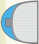
The Dura Glide features an integrated rubber rail reinforcement belt built into the rail, providing a maximum level of protection and maintains overall board performance.
